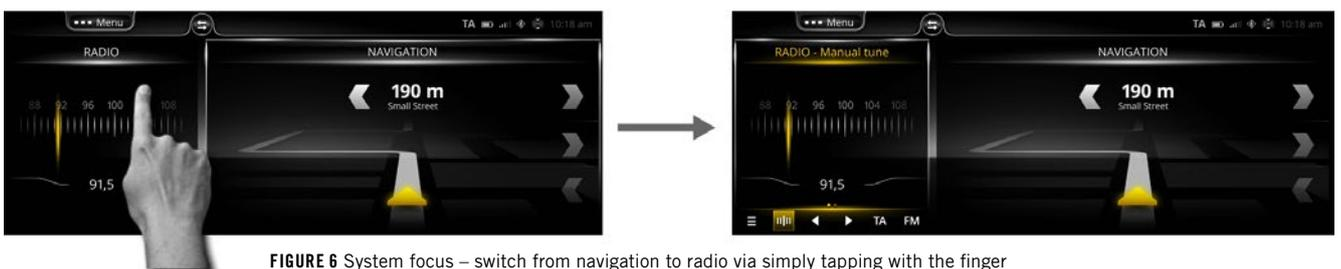
FIGURE 6 System focus – switch from navigation to radio via simply tapping with the finger
