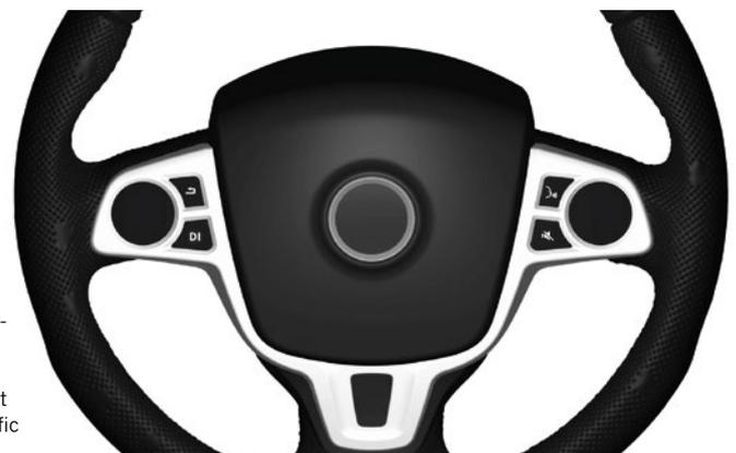
**FIGURE 1** Demonstrator steering wheel – the left input device offers full access to the functions, the right input device is dedicated to specific infotainment functions
