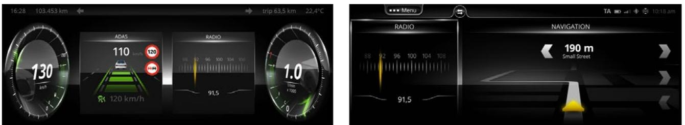
FIGURE 5 Radio app extension from CID (left) to ICD or HUD (right)
