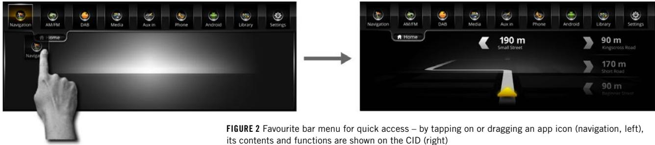
**FIGURE 2** Favourite bar menu for quick access – by tapping on or dragging an app icon (navigation, left), its contents and functions are shown on the CID (right)
