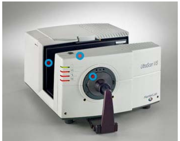
Figure 3-12. Hunter Lab UltraScan Spectrophotometer
