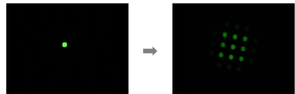
Figure 1-5. Individual light dot multiplied by 2-dimensional anti-sparkle grating [Courtesy of 3M]
