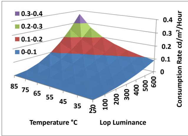
**Figure 2.1-2.** Luminance Consumption Rate as a Function of Temperature and Operational White Luminance
