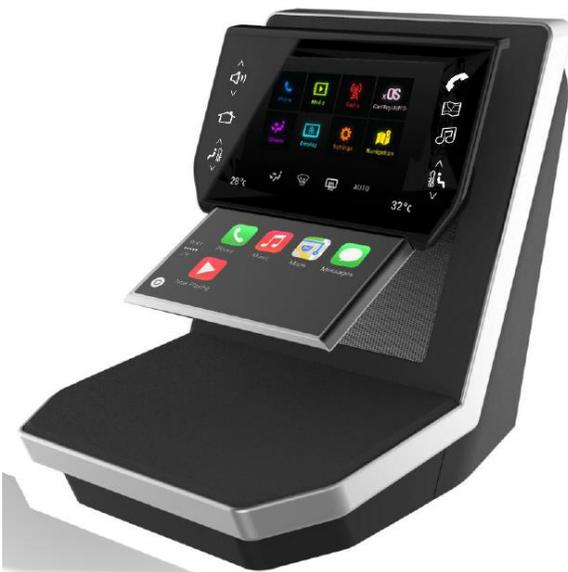
**Figure 4-1.** Dual OLED Demonstrator
