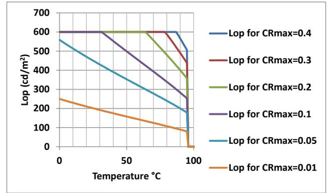
**Figure 2.2-1.**  $L_{op}$  versus Temperature for Different CRs
