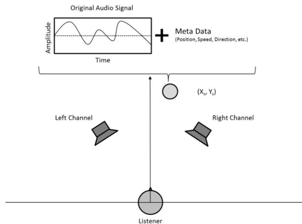
Figure 3: Virtual sound source (based on Sladeczek 2014)
