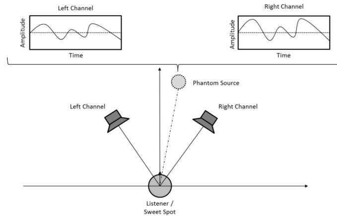
Figure 2: Phantom sound source (based on Sladeczek 2014)
