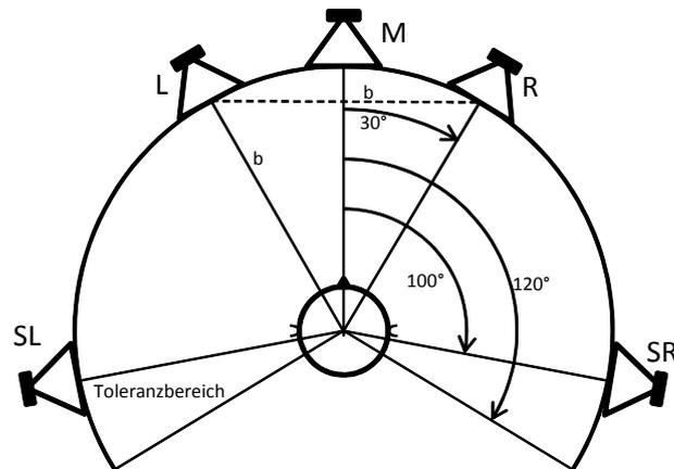
Figure 1: Surround System Setup. Based on (Rumsey, 2001)
