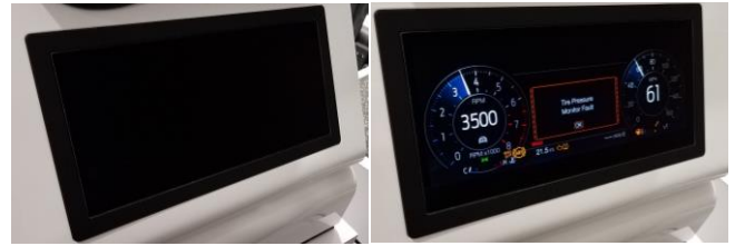
Figure 6-1. Display “Off”, Maximum Lens Dimming (Left) and Display “On” Minimum Lens Dimming Right
