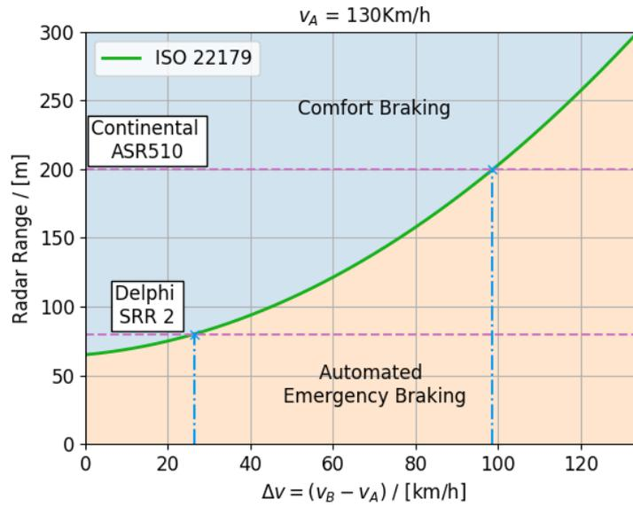
Figure 2: Closing speed ( $\Delta v$ ) variations with regard to range depicted by the radar sensor for a certain vehicle-A speed,  $v_A = 130 \text{ Km/h}$  corresponding to different braking profiles – (1) Comfort Braking, (2) Braking as per ISO 22179 standard, (3) Automated Emergency Braking.
