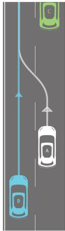
Figure 1: A driver-initiated automated lane change performed by the ego-vehicle (A) with fast approaching vehicle (B) in the adjacent lane.
