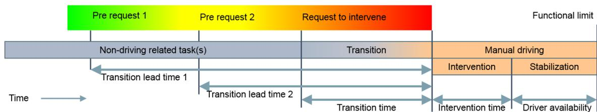
Figure 2 In case of a standard a functional limit an HMI cascade of 2 pre-requests with rising priorities develops over time. While the order in sequence of the cascade remains the same, the temporal organization may change due to unexpected events after the initial detection of the functional limit. The HMI cascade is designed to mitigate the dilemma when monitoring the driver status to increase system acceptance and maintains safe operation for standard takeover situations.
