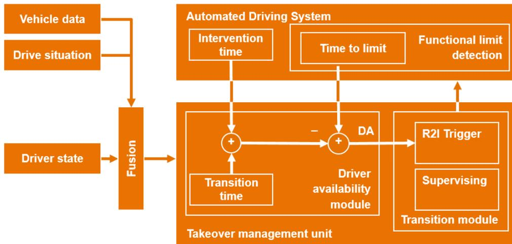
Figure 3 The takeover management resides next to the automated driving system and complements its functionalities to become a complete level 3 system. Here not only the driving situation needs to be assessed constantly but also the driver's status in order to provide appropriate leeway when it comes to a standard functional limit. The model of the takeover process needs to be updated constantly with the incoming data in order to manage the takeover safe and in an acceptable manner.
