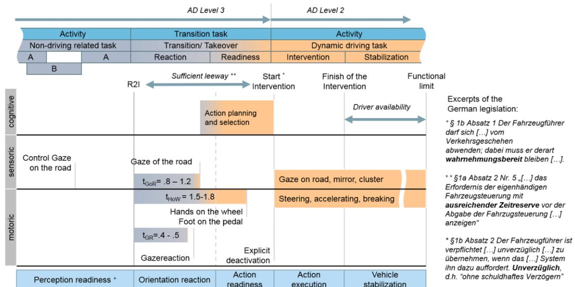
Figure 1 A Synopsis of the takeover at level 3 automation. While the driver pursue non-driving related activities a request to intervene (R2I) is issued when the driving system detects a functional limit. Drivers need to give up their activities immediately without due delay and become ready to drive manually. In standard situations enough leeway needs to be provided to allow for a safe and comfortable takeover.
